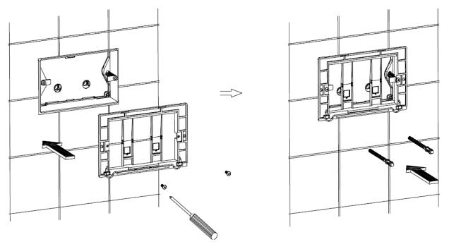
5. Once the rods are fully inserted, secure into position using the clips shown below, then push the rods to ensure free movement is achieved.
