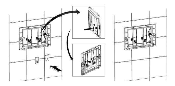
6. Attach the flush plate and click into position.
