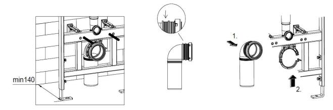
Option 2: Pan connector to be installed to the side
