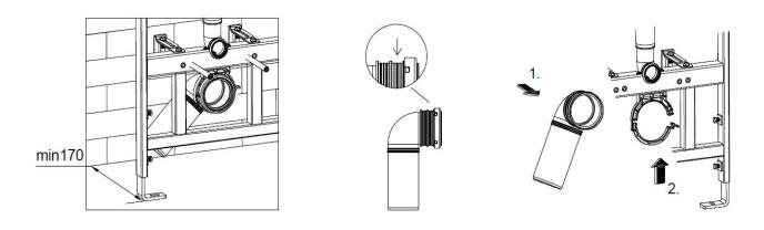
Below show the fixing width dimensions for the wall and floor screws, and the distance from the centre of the pan connector.
