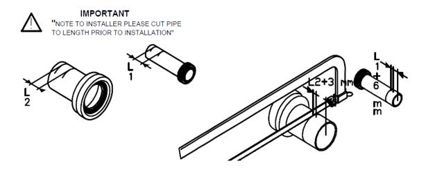
12. Prepare the flush pipe and pan connector ends removing any rough edges and create a small chamfer.
