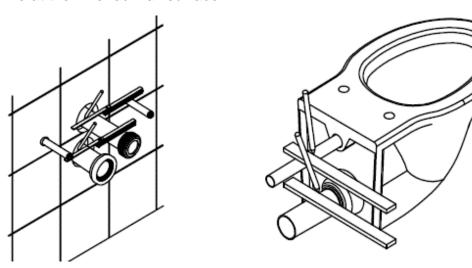
10. Remove from the frame and connect them to the flush hole and waste spigot on the rear of the toilet pan (Apply a small amount of washing up liquid to assist).
